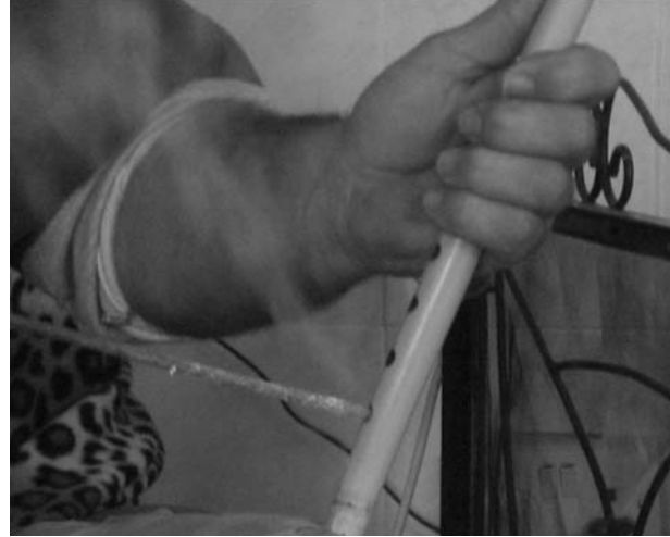
Boring the holes with a hot iron rod
